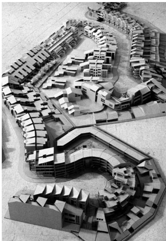
Housing Project on Curving Streets, Viewed from the South: (Left) Solar envelopes run continuously along the street, dropping to shadow fences only at front and back of lots; (Right) Housing designs under the envelope achieve a density range of 25 to 45 du/ac (62 to 111 du/ha), much higher than normal subdivision densities.
